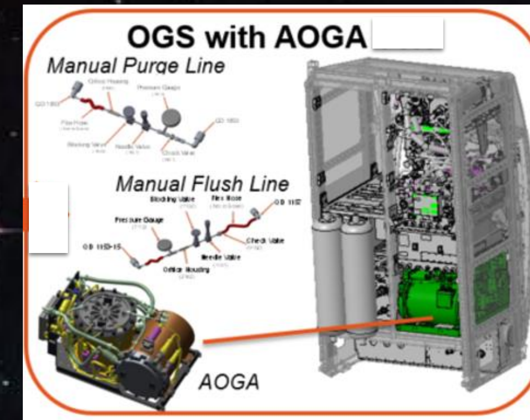
OGS rack with AOGA OHDA installed
