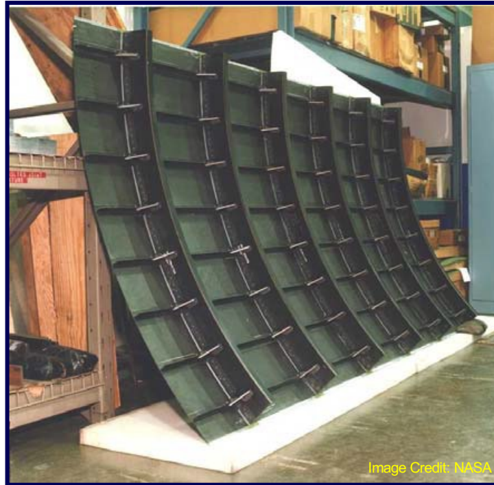
6 ft x 10 ft PETI-5/IM7 Skin Stringer Panel from High-Speed Research (HSR) Program
