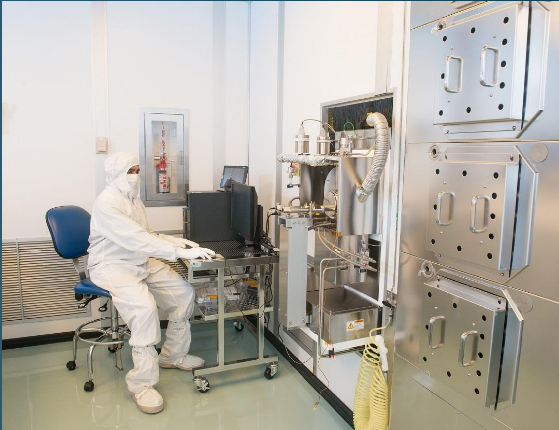
Oxidation and annealing furnaces; Silicon Dioxide Low Pressure Chemical Vapor Deposition System
