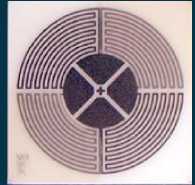
Heat Flux Thin Film Sensor Array to T=1000^{\circ}\text{C}
