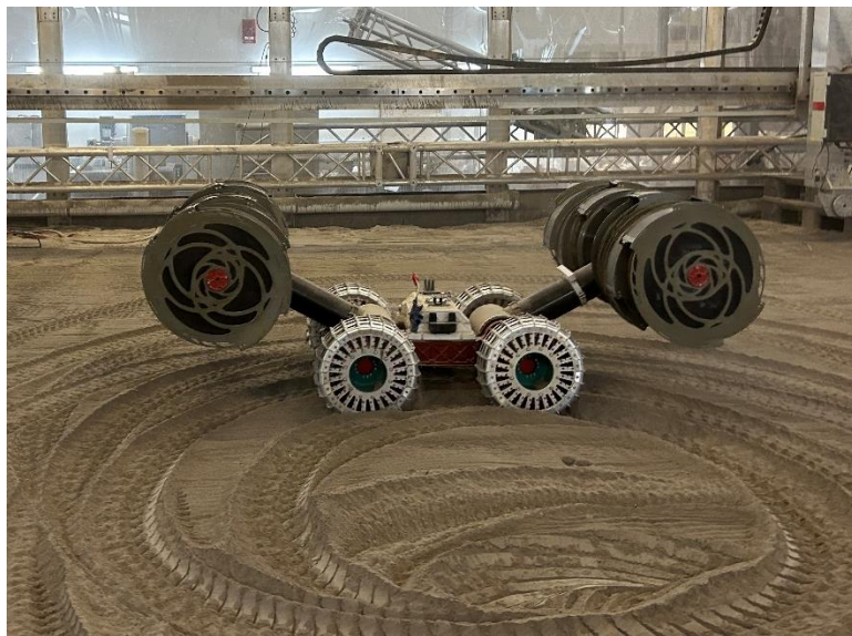
Fig. 11 RASSOR 2 excavator with IPEX concept test wheels.
