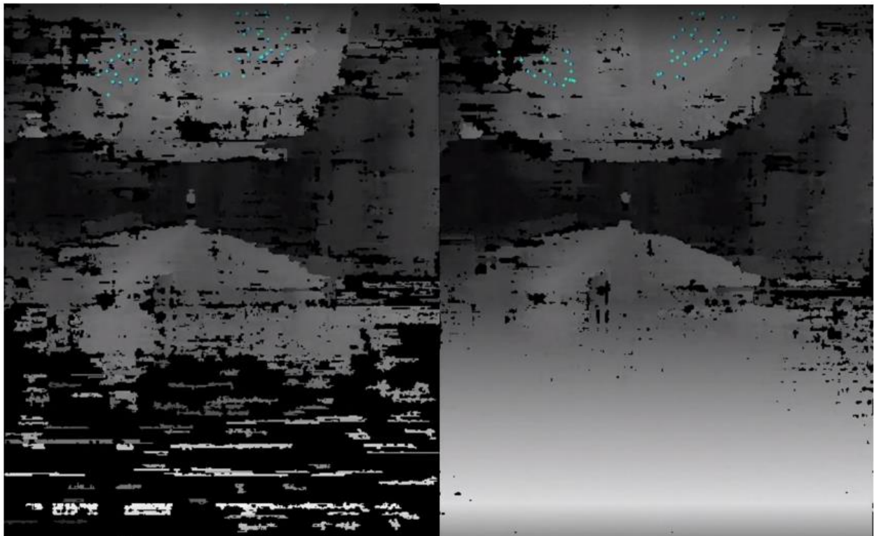
Fig. 29 Results of lost stereo calibration from an applied load with separated stereo camera units.
