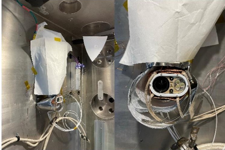
Fig. 34 IPEX camera installed in the ASSIST chamber.
