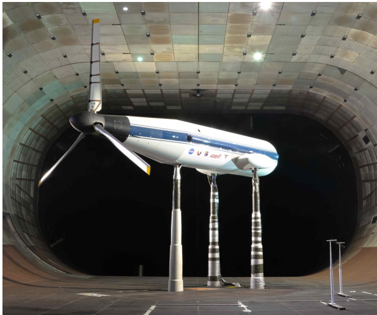
Fig. 1. TTR/699 installed in the NFAC 40- by 80-ft test section, 45-deg yaw.
