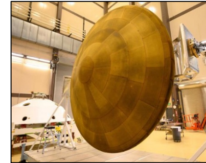
Mars Science Laboratory (MSL) heatshield with tiled PICA bonded by RTV560 [1].
