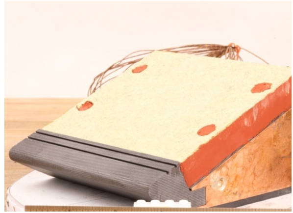
(d) 15° one-sided standard TPS wedge model with PICA material
