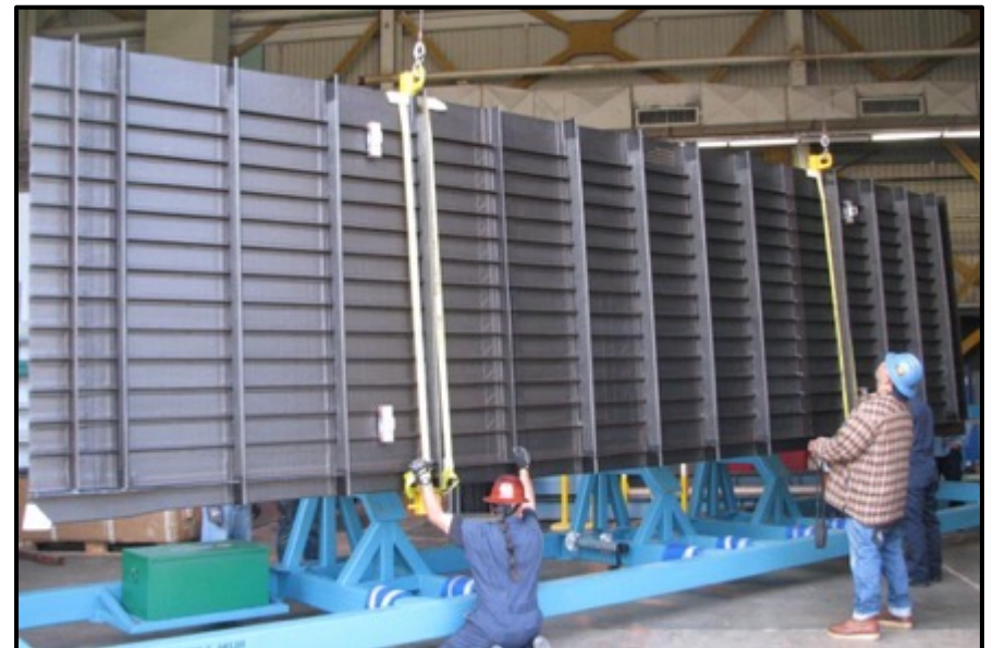
30-ft-long stitched panel with no fasteners 26
