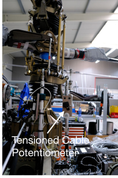
Fig. 6 Measurement of the control rod positions at the swashplate via tensioned cable potentiometers.
