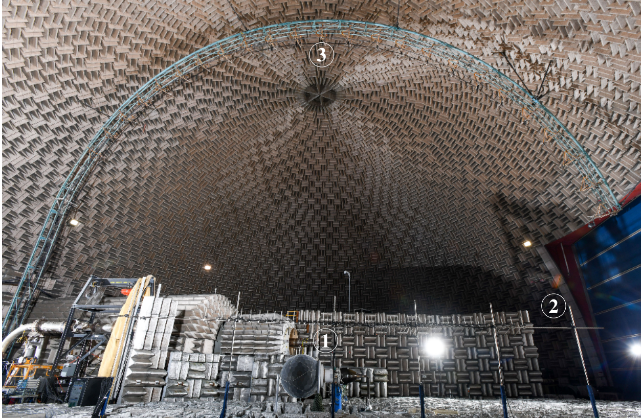
Figure 1. DART ①, sideline ② and overhead ③ arrays
