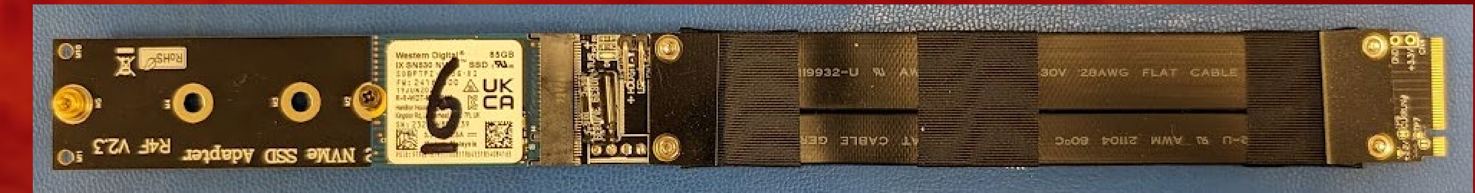
DUT mounted to passive PCIe adapter for testing.
