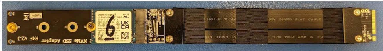
Fig. 1. DUT mounted to passive PCIe extender for testing.
