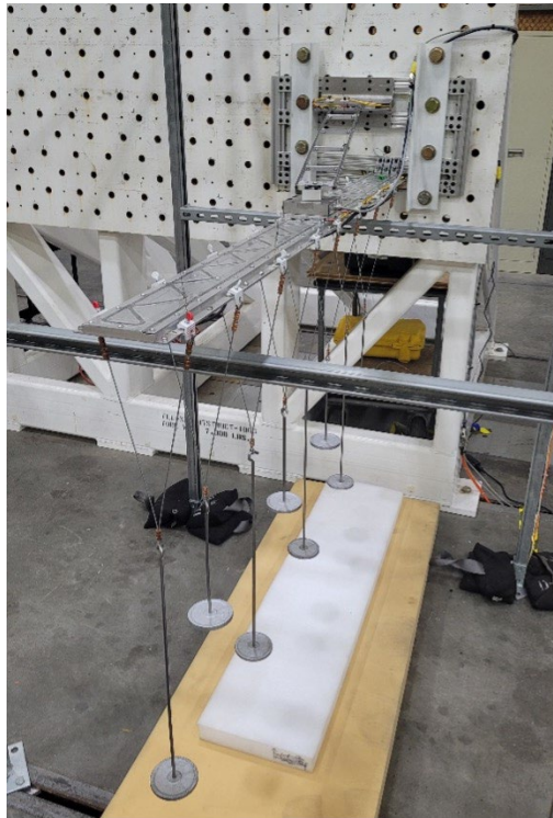
Figure 5. Mock Truss-Braced Wing on strongback.
