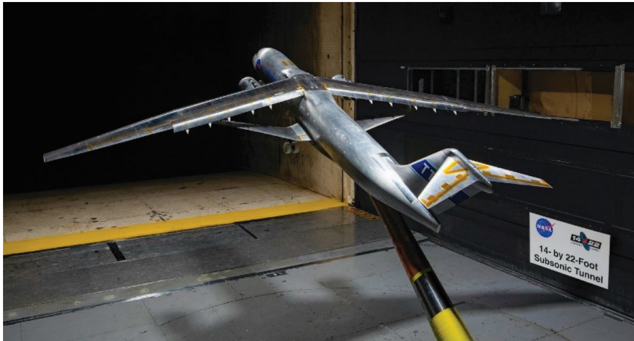
Figure 1. Truss-Braced Wing wind-tunnel test at NASA Langley Research Center (Hampton, Virginia).
