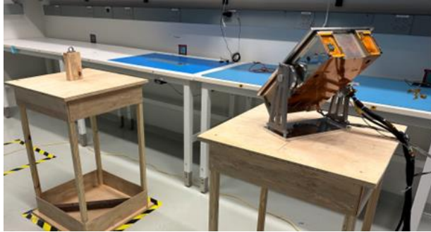
Figure 10 (a): Sample Calibration Setup with radiation source holder (left, gray hoop) and spacecraft rotated upside down(right)
