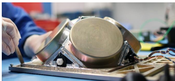
Figure 7: BurstCube instrument, detector heads (gold) visible on the mounting plate during integration (Photo credit: NASA/Sophia Roberts)
