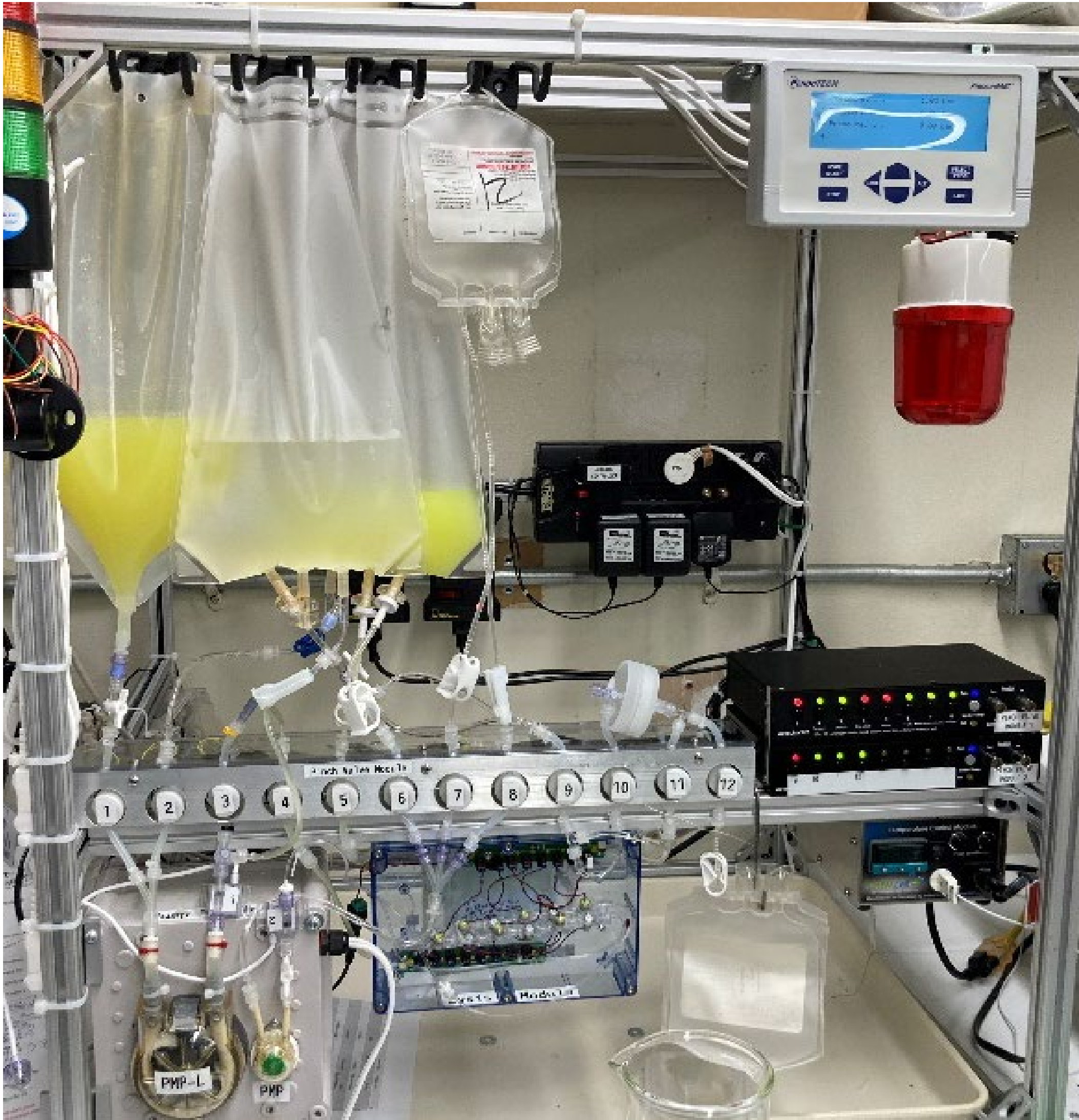
Figure 5: CO 2 -Based Manufacturing Prototype Platform Being Tested with E. coli emGFP
