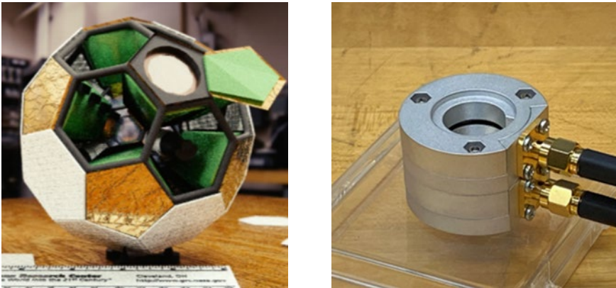
Left: Illustration of a configuration concept for multiple directional detectors. Right: Laboratory demonstrated directional detector.
