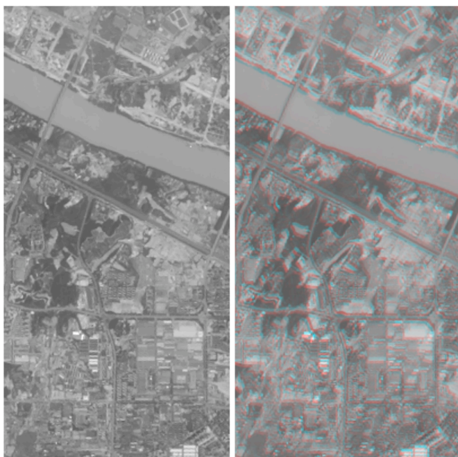
Fig. 2. Illustration of Level 1 TP Landsat geolocation differences between Collection 1 and Collection 2 for a panchromatic (0.50–0.68 \mu\text{m} ) 400 \times 200 15 m pixel subset extracted from a Landsat 8 OLI image acquired over a path/row where the mean longitude and latitude geolocation collection shifts are large (25.64 m and 36.75 m respectively, 44.81 m RMSD). Left: Collection 2 15 m panchromatic band shown as red, green, blue. Right: Collection 1, Collection 2, Collection 2 panchromatic band shown as red, green, blue, respectively. The misregistration between the Collection 1 and Collection 2 images is apparent in the magenta and cyan tones in the right image. The Landsat 8 OLI image was acquired September 2, 2020, over WRS-2 path 125/row 43 and the subset is centered at 24.348°N, 109.361°E, near Liuzhou, China.
