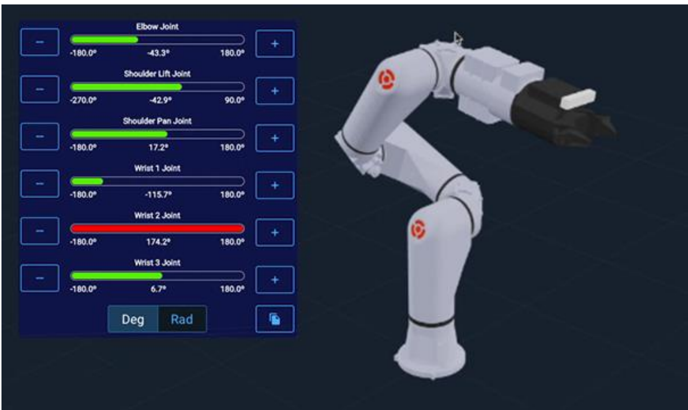
Figure 2: Motiv Space System's xLink robotic manipulator inside PickNik Robotic's MoveIt Pro software. (Source: https://picknik.ai/pro/scan-pick-and-place )
