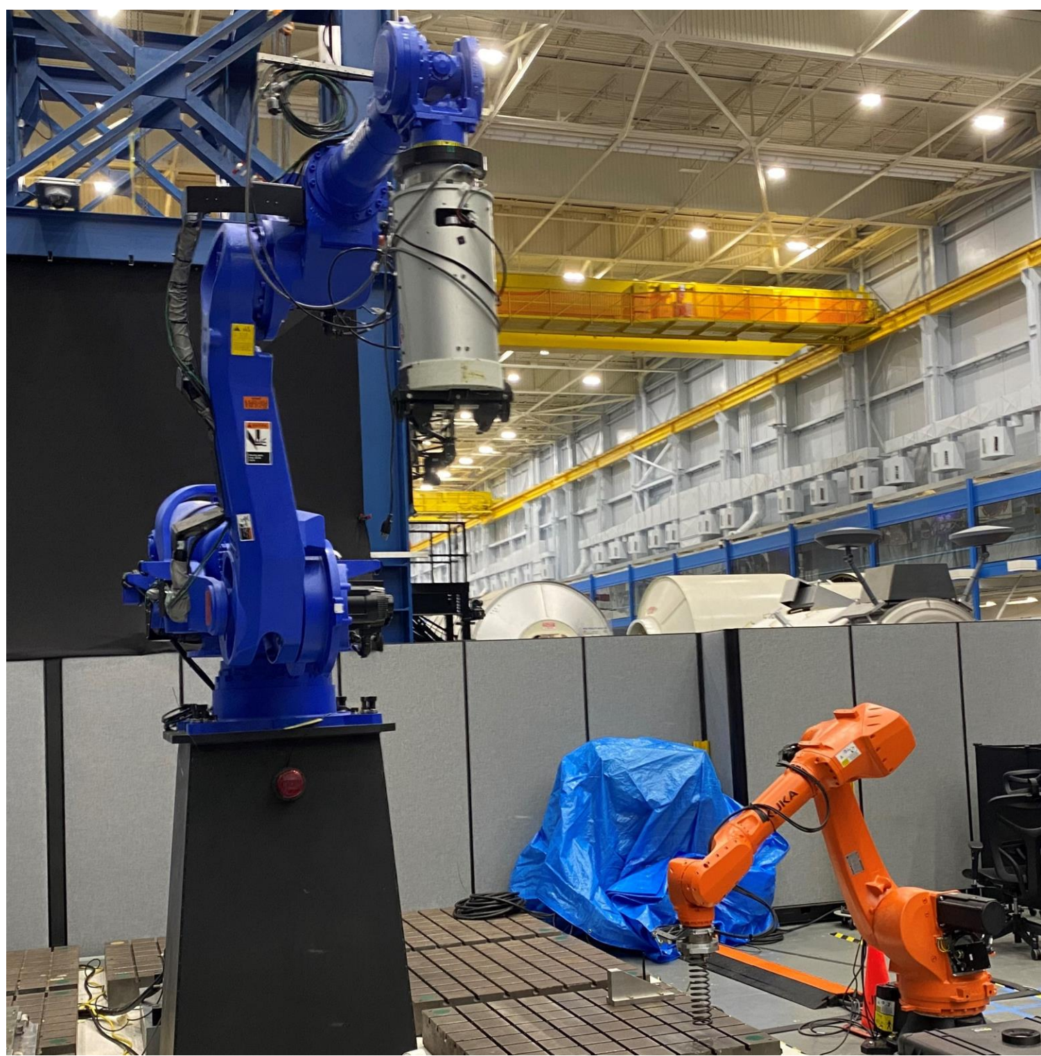
Figure 4: Medium and large payload robotic manipulators (Blue Yaskawa Motoman ES165 and Orange Kuka KR70). The large payload manipulator features the Orbital Replacement Unit/Tool Change-out Mechanism (OTCM) end effector used on the SPDM on ISS.
