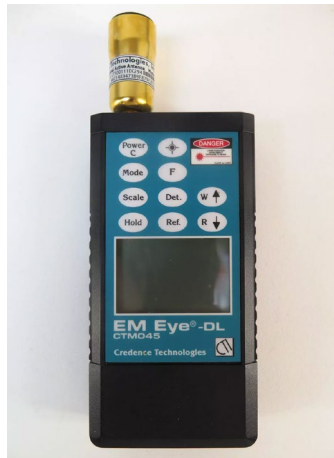
EM Eye-DL used to measure the magnitude of EMI generated during tribocharging
