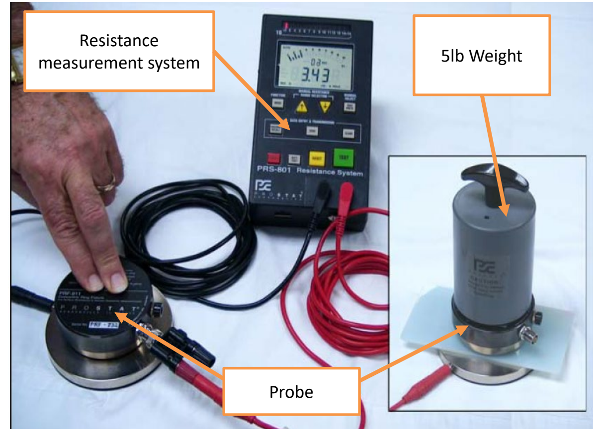
Example image of surface and volume resistance measurement apparatus. PRF-911 resistance probe placed on material for testing. 5lb weight placed on probe. PRS-801 resistance system used to capture measurements. [Image credit: Prostat Corporation]
