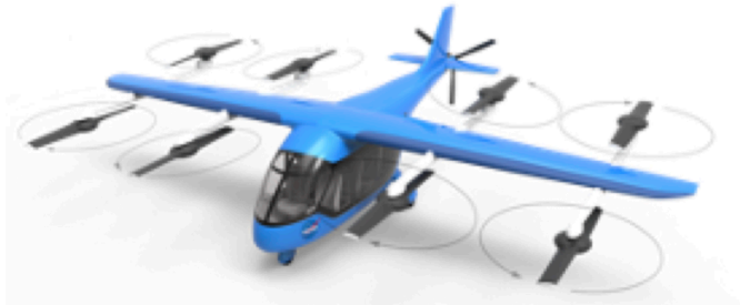
Fig. 2. Lift-Plus-Cruise (LPC) Aircraft
