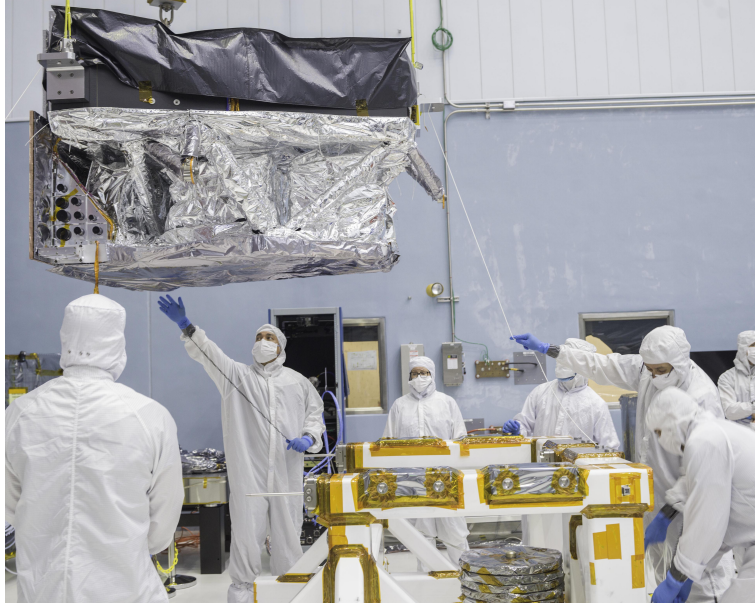
Figure 5. The Roman CGI has been delivered to Goddard and is awaiting installation into the IC. This image shows the unpacking of the CGI and installation in a holding fixture.
