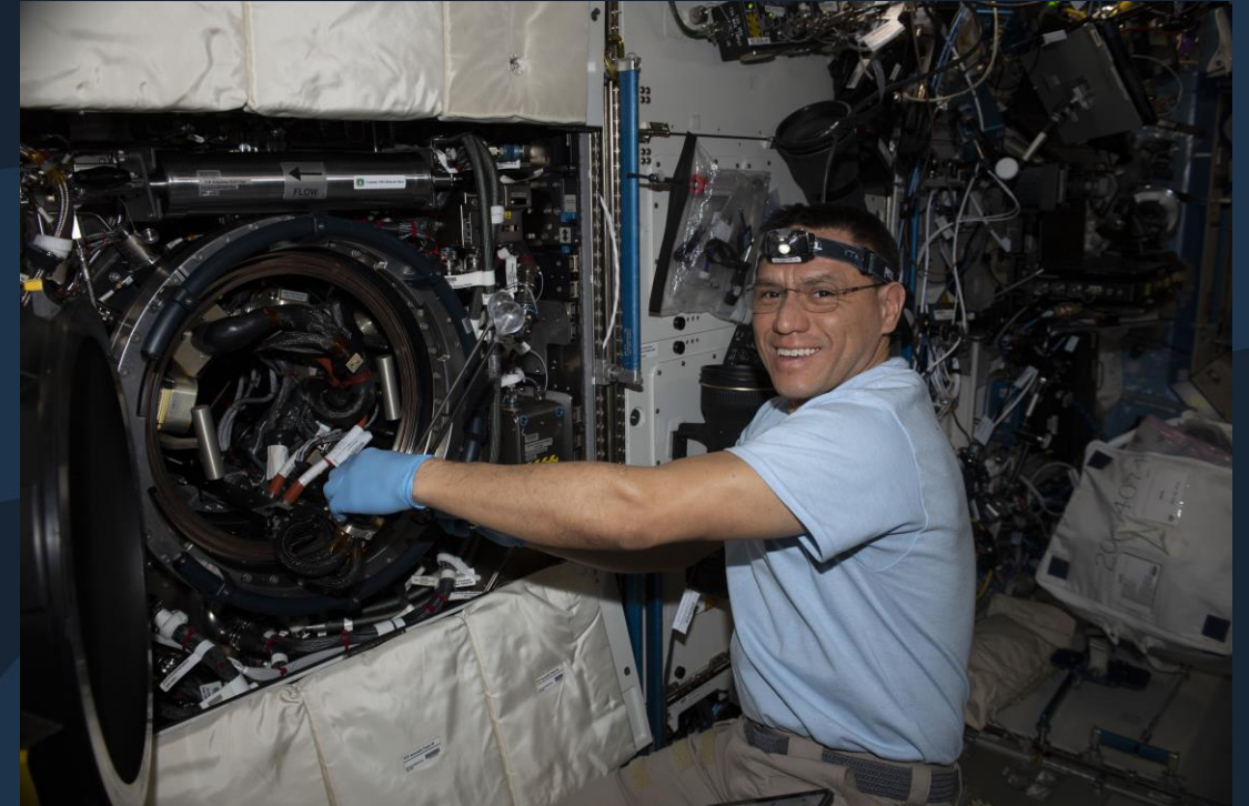
Pictured: NASA astronaut and Expedition 68 Flight Engineer Frank Rubio replaces experiment samples and research hardware inside the International Space Station's Combustion Integrated Rack for a study exploring how fires burn in weightlessness to improve fire safety techniques in space. Jan 2023. (Credit NASA ID iss068e043130)
