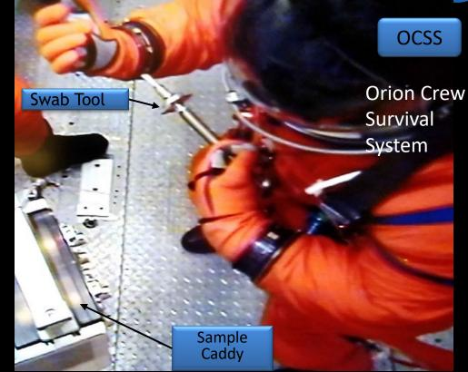
Sampling suit at vacuum in the 11 ft. chamber at Johnson Spac Center Internal suit pressure is 4.2 psia 29.6 Kpa)
