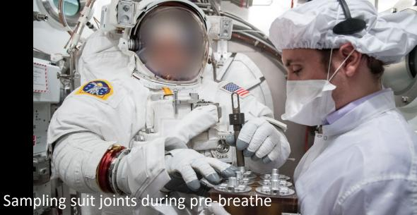
Sampling suit joints during pre-breathe Internal suit pressure is 4.2 psig (29.6 Kpa) above atmospheric pressure
