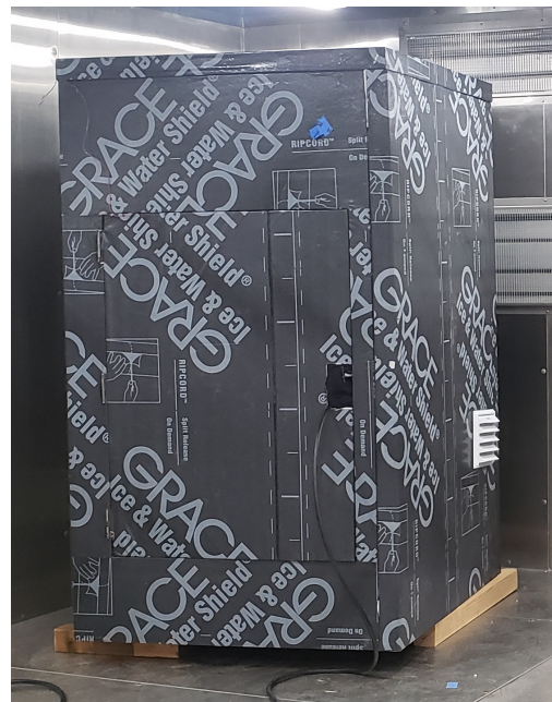
Figure E-21. Prototype GBO Enclosure during cold testing.
