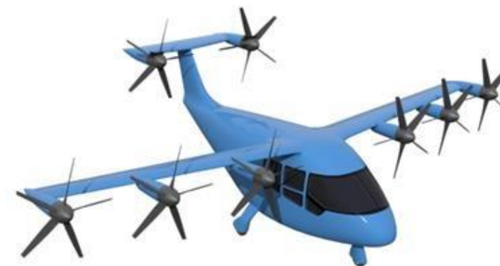
NASA Tiltwing Concept Vehicle (cruise configuration)
