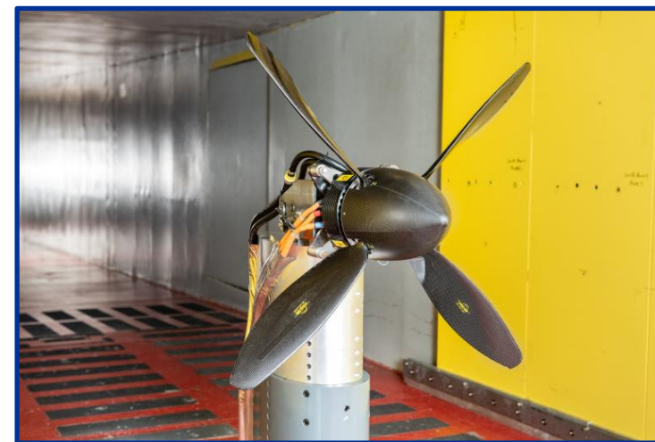
AAM Propeller Test Stand Installed in Icing Research Tunnel (IRT)
