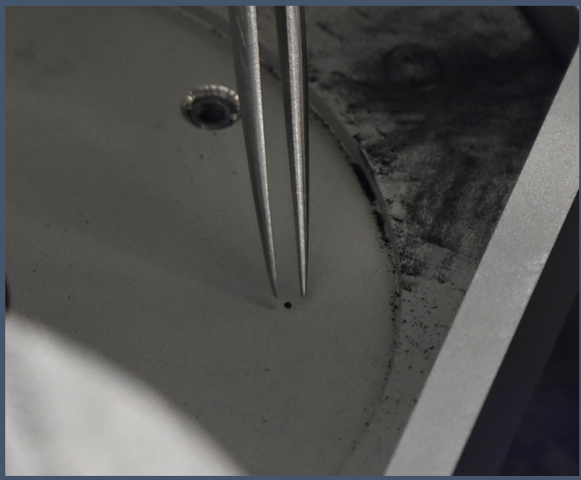
Particles on the micro to millimeter-size scale are more rounded and prone to jumping out of the tweezers grip. Precision curved-tip tweezers [Fig.3] were used to collect individual particles. It is necessary to grip these particle with as little force as possible.
