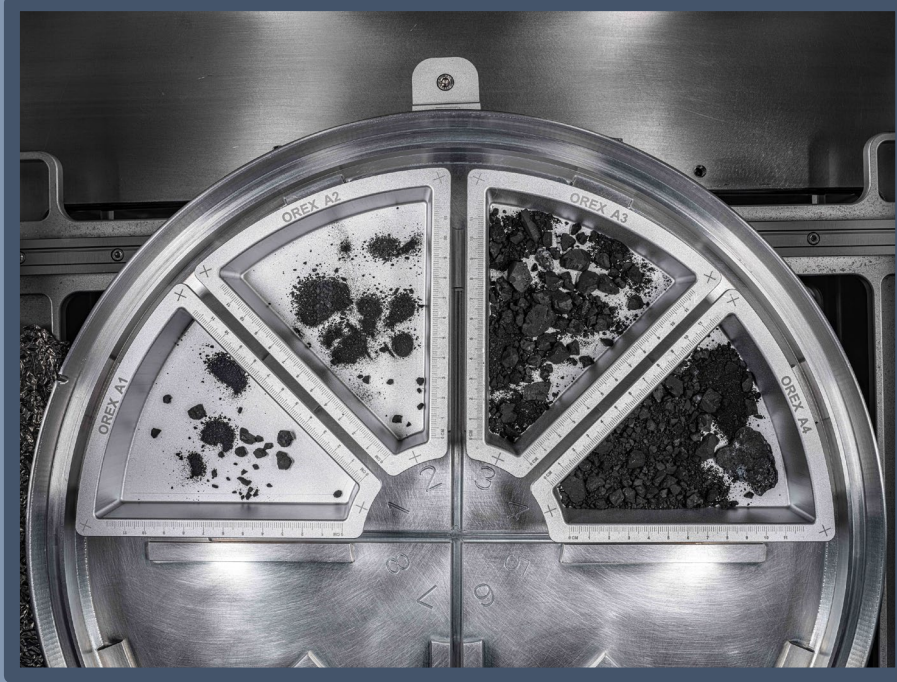
70.3g of material from within the TAGSAM head was extracted before it was fully disassembled; surpassing the mission mass requirement of at least 60 grams of material [3]. Photo Credit: NASA/Erika Blumenfeld & Joseph Aebersold
