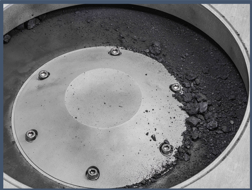
Bulk sample material on TAGSAM head deflector cone and mylar flap. Photo Credit: NASA/Erika Blumenfeld & Joseph Aebersold
