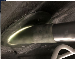
Nose cone composite structure proof tested
