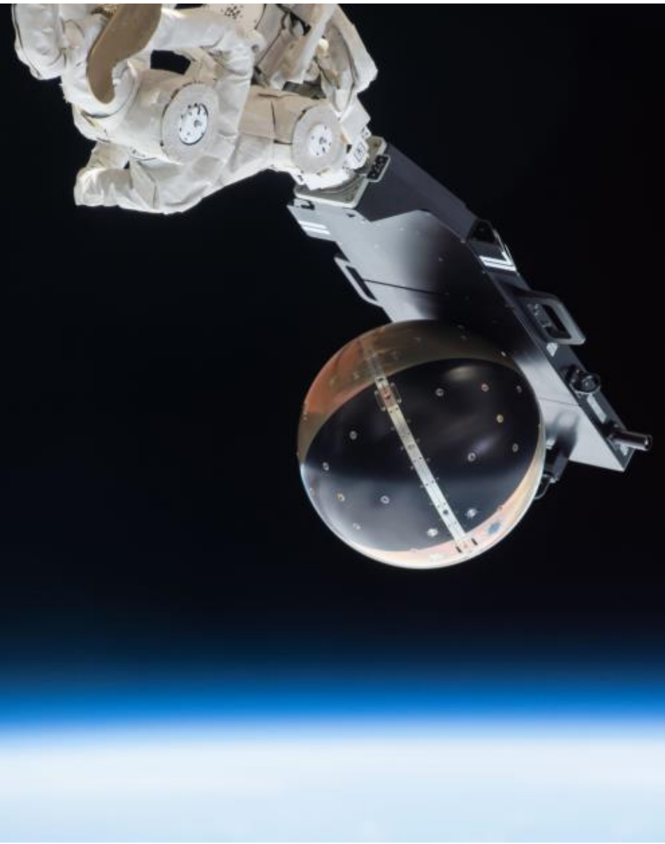
Left: Cyclops deployer with SpinSat preparing for release, Nov 2014
