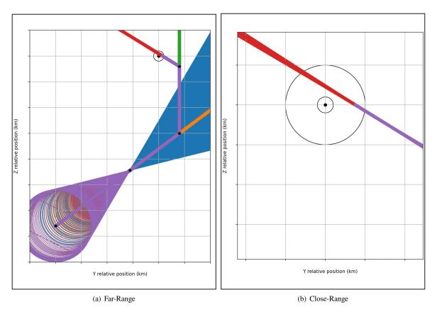
Fig. 6 Notional relative NRHO RPOD trajectory profile with anticipated trajectory dispersions
