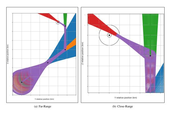
Fig. 8 Trajectory dispersions for an optimized navigation system given a fixed notional trajectory
