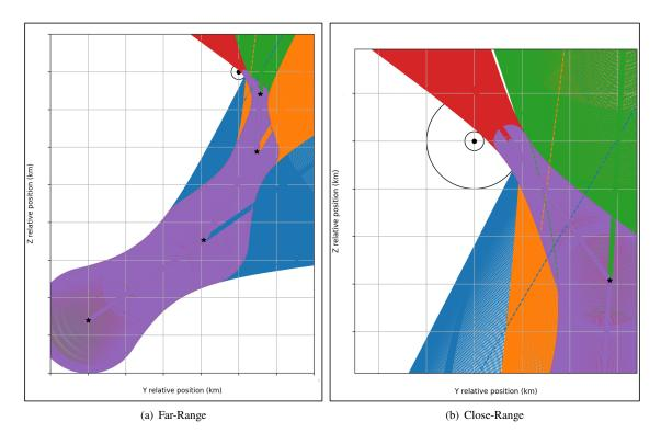
Fig. 10 Trajectory profile and dispersions for a co-optimized trajectory design and navigation system.
