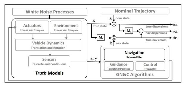
Fig. 2 Extracting GN&C Performance Metrics Using Monte Carlo Techniques
