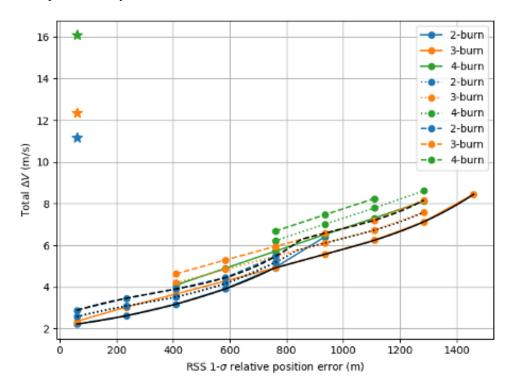
Fig. 12 Pareto front for navigation system requirement and trajectory design
