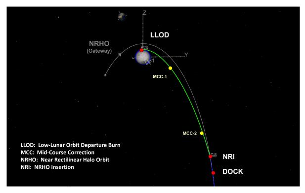
Fig. 3 Low Lunar Orbit to NRHO Rendezvous and Docking Profile
