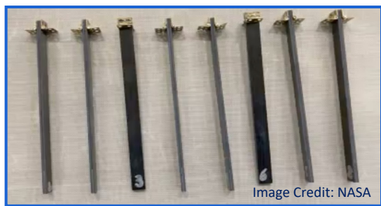
CNT Composite DCB Samples
