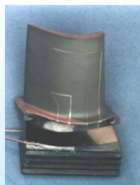
Pt- Pt/Rh temperature sensor to T=1200^{\circ}\text{C}
