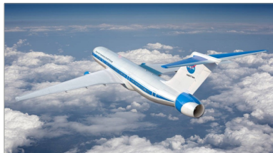
Type-II BLI example (Credit: NASA)
