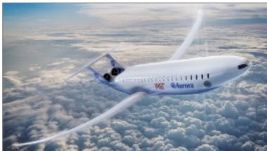
Type-I BLI example (Credit: NASA)
