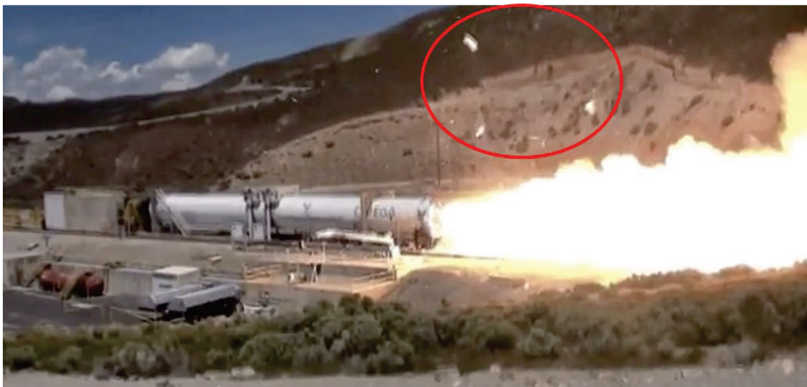
Figure 1. Nozzle Failure During the Omega SRM Test [ref. 13]
