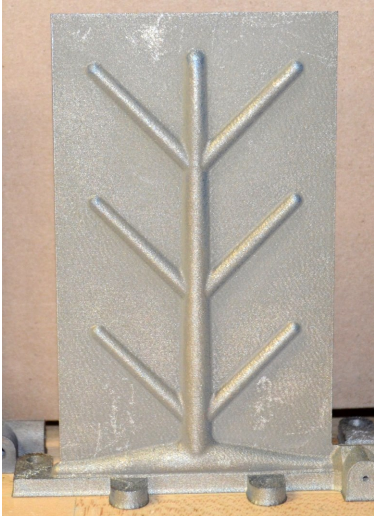
CP-Ti HPR Specimen
