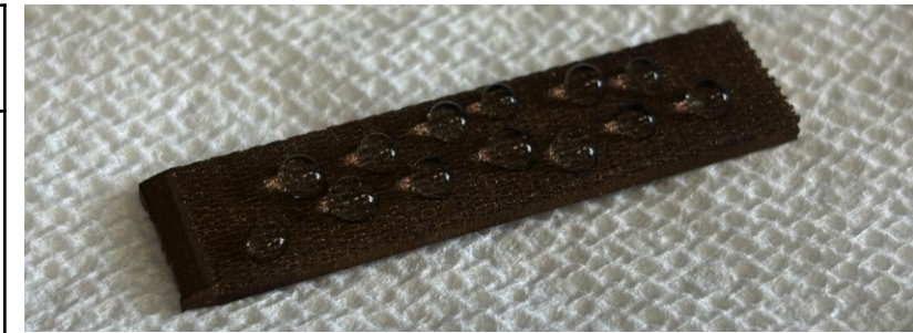
Example of a hydrophobic CP-Ti specimen
