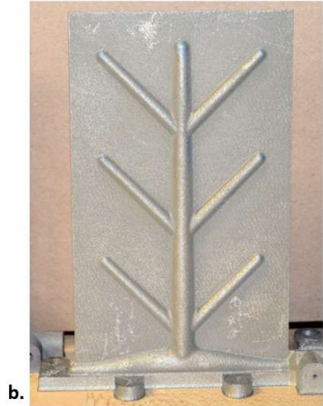
378 Figure 11: a. Annotated picture of set-up for the hydrogen peroxide oxidation treatment, b. Picture 379 of an untreated CP-Ti small-scale radiator.
