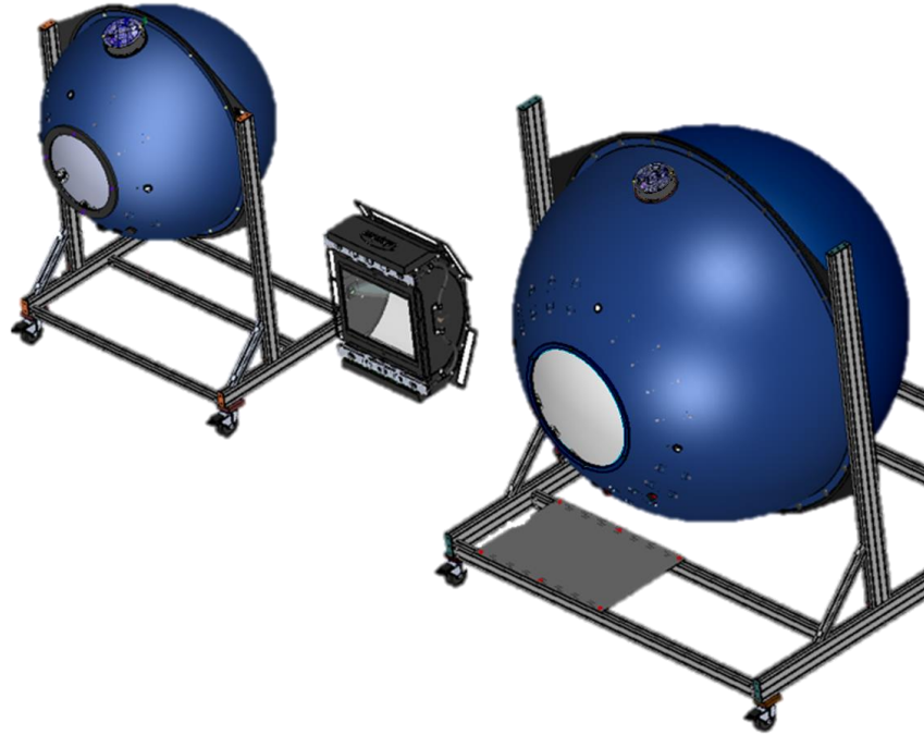
Figure 16: Contrasting CAD Models Showing Relative Size of a 40'' Diameter Integrating Sphere, the LVIS System, and a 65'' Diameter Integrating Sphere
