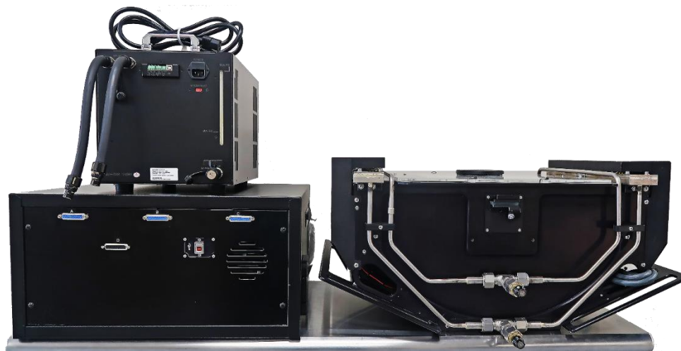
Figure 2: FPI II Demonstration Unit; including demo chiller (top left), source electronics module, and LVIS
