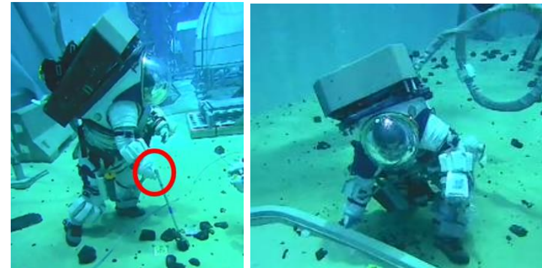
Increased physical demand (hand fatigue) due to glove pressurization
