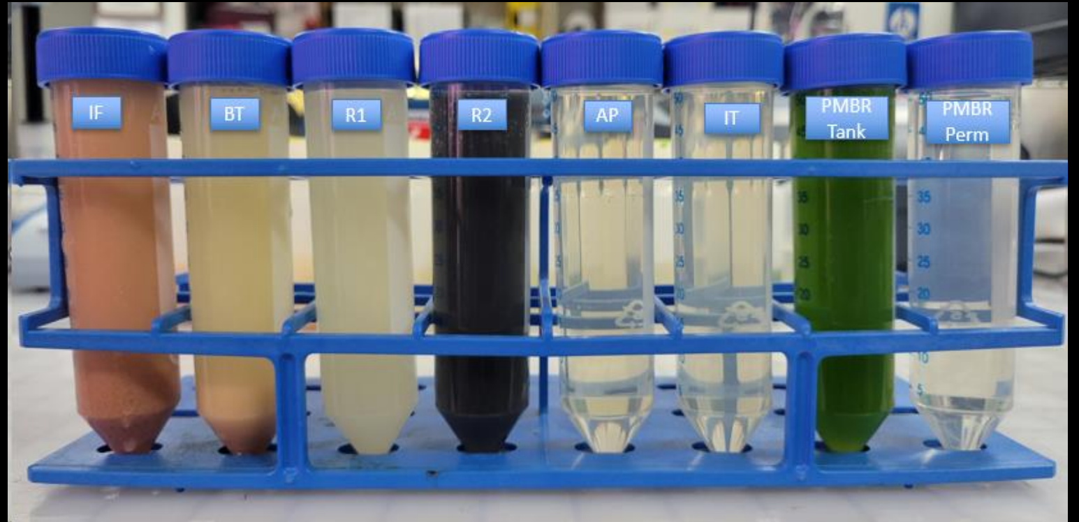
APMBR Samples pre-centrifugation. From left to right: Influent tank (IF), Buffer Tank (BT), Reactor Tank 1 (R1), Reactor Tank 2 (R2), Anaerobic Permeate (AP) Intermediary Tank (IT), PMBR tank, and PMBR Permeate (PP).
