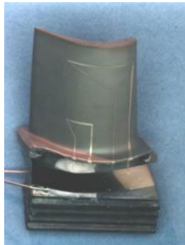
Pt- Pt/Rh temperature sensor to T=1200^{\circ}\text{C}
