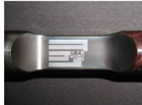
PdCr thin film strain gauge applied to a material sample for disk life fatigue testing
