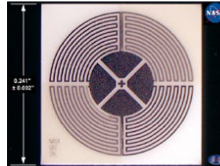
Heat Flux Sensor Array to T=1000^{\circ}\text{C}
