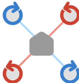
Figure 1: An X-Frame quadcopter UAV design. The rotors, which will be used for the propellers, are represented by the blue and red arrows.
