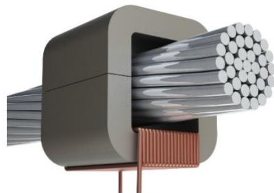
Figure 5: An Illustration of the Energy Harvester (Image credit: Muñoz-Gómez) [51].
