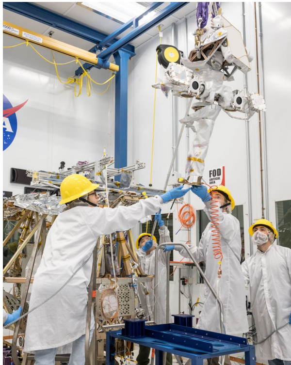
Fig. 7: VIPER mast installation
