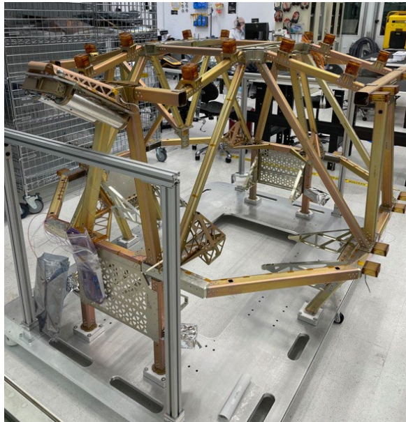
Fig. 4: VIPER upper frame assembly
