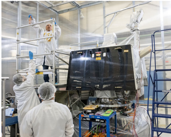
Fig. 10: VIPER undergoing Sine-Vibe testing.
