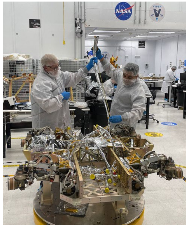
Fig. 3: Wheel suspension system installation
