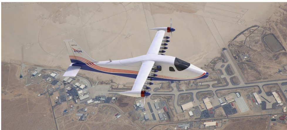
Figure 4 – Rendering of the X-57 in the Mod III configuration in flight.
