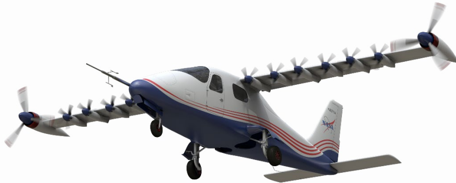
Figure 5 – Rendering of the X-57 in the Mod IV configuration with the high-lift propellers deployed.
