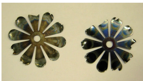
1950's era RPC Reed Valves After 15 sec. Operation in Gas Turbine
