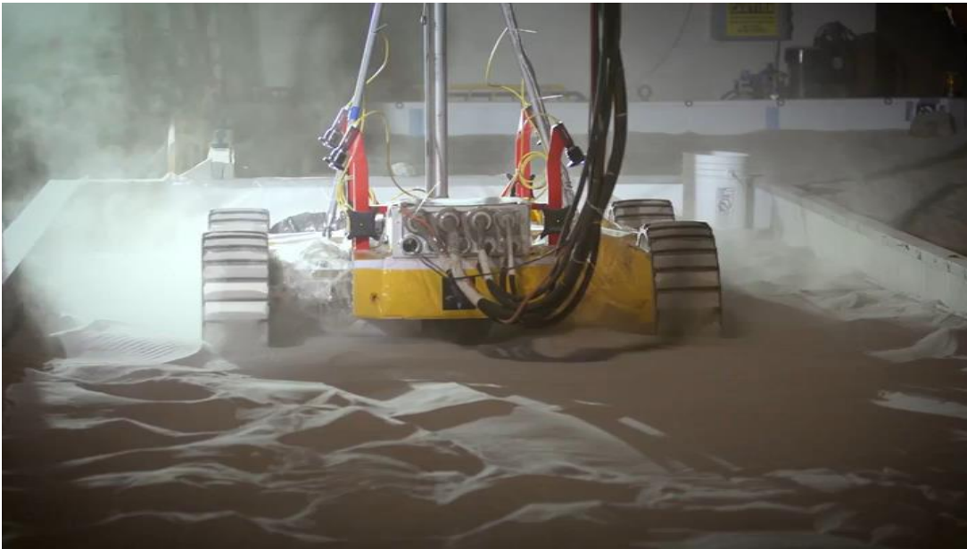
Rigid wheel testing of NASA's VIPER and JPL's CADRE
