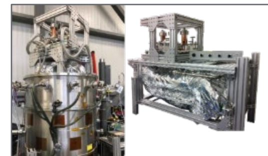
20W 20K Cryocooler in Cleanroom
