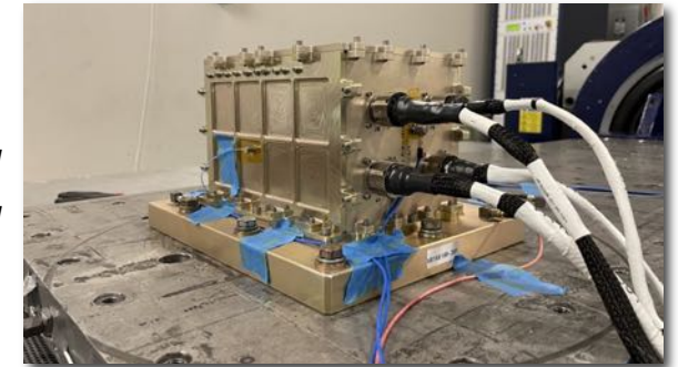
Avionics box during vibration testing
