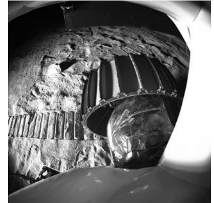
Appearance of VIPER rover wheel and tracks
