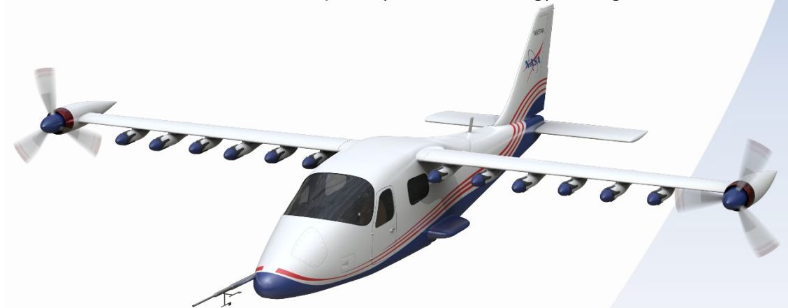
X-57 Mod IV in High-Speed (Cruise) Configuration (Identical to X-57 Mod III)
