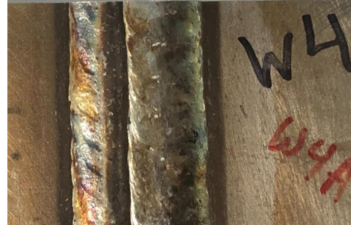
W1: Root: GTAW Cover: FCAW KJ -452°F : 58.4ksiVin
