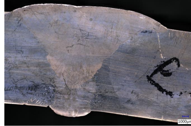
W4: Root: GTAW Cover: FCAW KJ -452°F : 103.1 ksiVin
