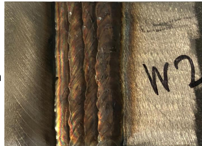
W2: Root: GTAW Cover: GTAW KJ -452°F : 154.2ksiVin
