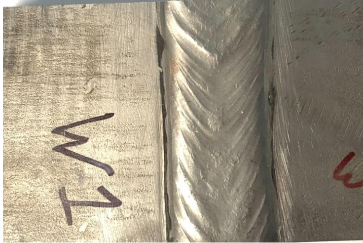
W1: Root: GTAW Cover: FCAW KJ -452°F : 58.4ksiVin
