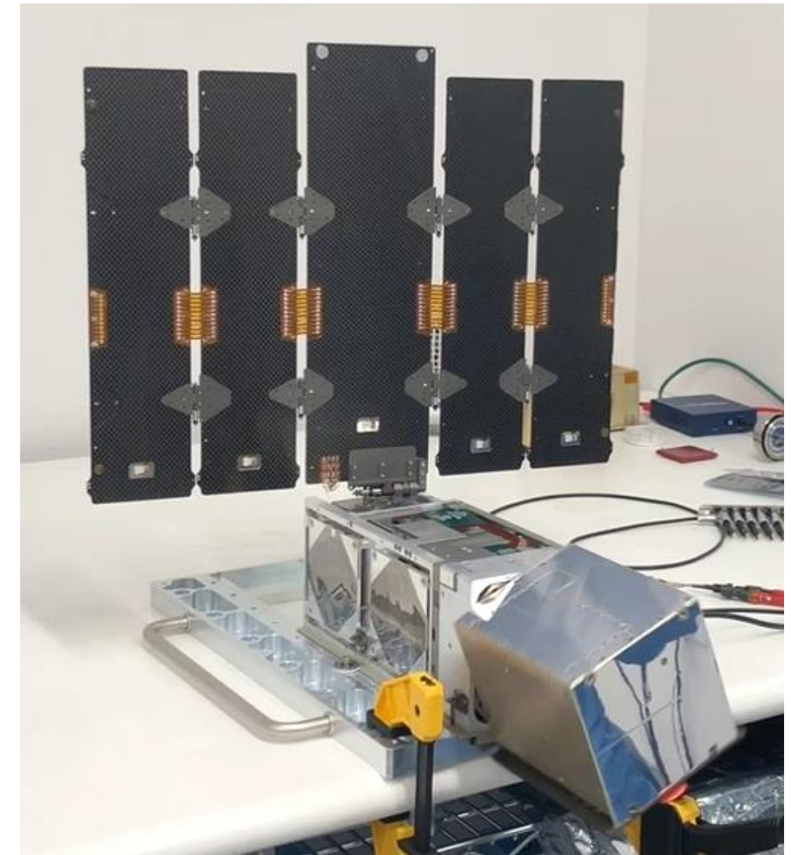
The primary microwave radiometer payload continuously spins throughout the orbit of the TROPICS satellites
